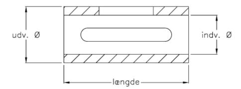
Description = 9/14Internal diameter = 9Length = 26Outer diameter = 14
